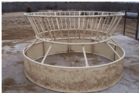
Sheeted-bottom ring with a basket Total bale waste = 5.5%
